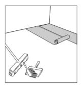
After thoroughly cleaning the subfloor, you should install a foam underlay (unless your product has a pre-attached pad). Run the foam underlay in the same direction as the flooring planks. The underlay should be butted side-by-side with no overlap. Tape seams together. If you are installing over a concrete suboor, a 6-mil poly (plastic sheeting) is to be installed under the foam underlay.
