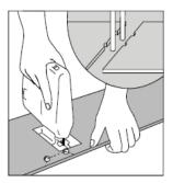
Holes for pipes: measure the diameter of the pipe and drill a hole that is 7/8" / 20 mm larger. Saw off a piece as shown in the figure and lay the board in place on the floor. Then lay the sawed-off piece in place.
